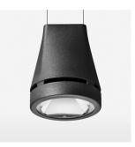
Suspended luminaire with LED, rated life of the LED L80/B10 > 50000 h, colour rendering index CRI > 70, chromaticity tolerance 2 SDCM (initial), reflector with circular light distribution pattern, reflector pure aluminium 99,99% in MIRO-Silver®, canopy sheet steel, powder-coated, luminaire head die-cast aluminium, powder-coated, black
