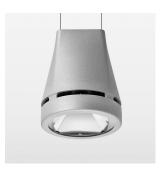
Suspended luminaire with LED, rated life of the LED L80/B10 > 50000 h, colour rendering index CRI > 70, chromaticity tolerance 2 SDCM (initial), reflector with circular light distribution pattern, reflector pure aluminium 99,99% in MIRO-Silver®, canopy sheet steel, powder-coated, luminaire head die-cast aluminium, powder-coated, silver
