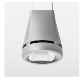
Suspended luminaire with LED, rated life of the LED L80/B10 > 50000 h, colour rendering index CRI > 80, chromaticity tolerance 2 SDCM (initial), reflector with circular light distribution pattern, reflector pure aluminium 99,99% in MIRO-Silver®, canopy sheet steel, powder-coated, luminaire head die-cast aluminium, powder-coated, silver
