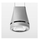
Suspended luminaire with LED, rated life of the LED L80/B10 > 50000 h, colour rendering index CRI > 80, chromaticity tolerance 2 SDCM (initial), reflector with circular light distribution pattern, reflector pure aluminium 99,99% in MIRO-Silver®, canopy sheet steel, powder-coated, luminaire head die-cast aluminium, powder-coated, silver
