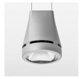
Suspended luminaire with LED, rated life of the LED L80/B10 > 50000 h, colour rendering index CRI > 70, chromaticity tolerance 2 SDCM (initial), reflector with circular light distribution pattern, reflector pure aluminium 99,99% in MIRO-Silver®, luminaire head die-cast aluminium, powder-coated, silver
