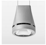
Suspended luminaire with LED, rated life of the LED L80/B10 > 50000 h, colour rendering index CRI > 70, chromaticity tolerance 2 SDCM (initial), reflector with circular light distribution pattern, reflector pure aluminium 99,99% in MIRO-Silver®, luminaire head die-cast aluminium, powder-coated, cilver
