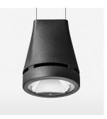
Suspended luminaire with LED, rated life of the LED L80/B10 > 50000 h, colour rendering index CRI > 82, chromaticity tolerance 2 SDCM (initial), reflector with circular light distribution pattern, reflector pure aluminium 99,99% in MIRO-Silver®, luminaire head die-cast aluminium, powder-coated, black
