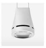
Suspended luminaire with LED, rated life of the LED L80/B10 > 50000 h, colour rendering index CRI > 80, chromaticity tolerance 2 SDCM (initial), reflector with oval light distribution pattern, reflector pure aluminium 99,99% in MIRO-Silver®, luminaire head die-cast aluminium, powder-coated, white
