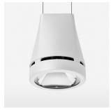
Suspended luminaire with LED, rated life of the LED L80/B10 > 50000 h, colour rendering index CRI > 82, chromaticity tolerance 2 SDCM (initial), reflector with circular light distribution pattern, reflector pure aluminium 99,99% in MIRO-Silver®, luminaire head die-cast aluminium, powder-coated, white
