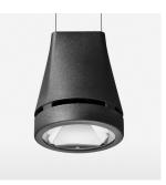
Suspended luminaire with LED, rated life of the LED L80/B10 > 50000 h, colour rendering index CRI > 90, chromaticity tolerance 2 SDCM (initial), reflector with circular light distribution pattern, reflector pure aluminium 99,99% in MIRO-Silver®, luminaire head die-cast aluminium, powder-coated, black
