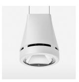
Suspended luminaire with LED, rated life of the LED L80/B10 > 50000 h, colour rendering index CRI > 70, chromaticity tolerance 2 SDCM (initial), reflector with circular light distribution pattern, reflector pure aluminium 99,99% in MIRO-Silver®, luminaire head die-cast aluminium, powder-coated, white
