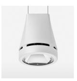
Suspended luminaire with LED, rated life of the LED L80/B10 > 50000 h, colour rendering index CRI > 90, chromaticity tolerance 2 SDCM (initial), reflector with circular light distribution pattern, reflector pure aluminium 99,99% in MIRO-Silver®, luminaire head die-cast aluminium, powder-coated, white
