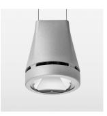
Suspended luminaire with LED, rated life of the LED L80/B10 > 50000 h, colour rendering index CRI > 70, chromaticity tolerance 2 SDCM (initial), reflector with circular light distribution pattern, reflector pure aluminium 99,99% in MIRO-Silver®, luminaire head die-cast aluminium, powder-coated, silver
