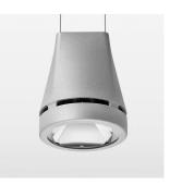
Suspended luminaire with LED, rated life of the LED L80/B10 > 50000 h, colour rendering index CRI > 90, chromaticity tolerance 2 SDCM (initial), reflector with circular light distribution pattern, reflector pure aluminium 99,99% in MIRO-Silver®, luminaire head die-cast aluminium, powder-coated, silver
