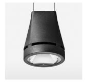
Suspended luminaire with LED, rated life of the LED L80/B10 > 50000 h, colour rendering index CRI > 80, chromaticity tolerance 2 SDCM (initial), reflector with circular light distribution pattern, reflector pure aluminium 99,99% in MIRO-Silver®, luminaire head die-cast aluminium, powder-coated, black
