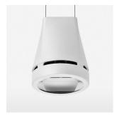
Suspended luminaire with LED, rated life of the LED L80/B10 > 50000 h, colour rendering index CRI > 90, chromaticity tolerance 2 SDCM (initial), reflector with oval light distribution pattern, reflector pure aluminium 99,99% in MIRO-Silver®, luminaire head die-cast aluminium, powder-coated, white, separate driver unit
