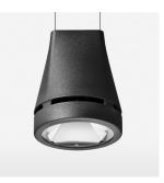
Suspended luminaire with LED, rated life of the LED L80/B10 > 50000 h, colour rendering index CRI > 80, chromaticity tolerance 2 SDCM (initial), reflector with circular light distribution pattern, reflector pure aluminium 99,99% in MIRO-Silver®, luminaire head die-cast aluminium, powder-coated, black, separate driver unit
