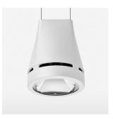
Suspended luminaire with LED, rated life of the LED L80/B10 > 50000 h, colour rendering index CRI > 90, chromaticity tolerance 2 SDCM (initial), reflector with circular light distribution pattern, reflector pure aluminium 99,99% in MIRO-Silver®, luminaire head die-cast aluminium, powder-coated, white, separate driver unit
