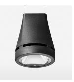
Suspended luminaire with LED, rated life of the LED L80/B10 > 50000 h, colour rendering index CRI > 90, chromaticity tolerance 2 SDCM (initial), reflector with circular light distribution pattern, reflector pure aluminium 99,99% in MIRO-Silver®, luminaire head die-cast aluminium, powder-coated, black, separate driver unit
