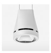
Suspended luminaire with LED, rated life of the LED L80/B10 > 50000 h, colour rendering index CRI > 90, chromaticity tolerance 2 SDCM (initial), reflector with circular light distribution pattern, reflector pure aluminium 99,99% in MIRO-Silver®, canopy sheet steel, powder-coated, luminaire head die-cast aluminium, powder-coated, white
