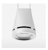
Suspended luminaire with LED, rated life of the LED L80/B10 > 50000 h, colour rendering index CRI > 70, chromaticity tolerance 2 SDCM (initial), reflector with oval light distribution pattern, reflector pure aluminium 99,99% in MIRO-Silver®, canopy sheet steel, powder-coated, luminaire head die-cast aluminium, powder-coated, white
