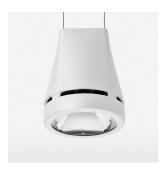
Suspended luminaire with LED, rated life of the LED L80/B10 > 50000 h, colour rendering index CRI > 82, chromaticity tolerance 2 SDCM (initial), reflector with circular light distribution pattern, reflector pure aluminium 99,99% in MIRO-Silver®, canopy sheet steel, powder-coated, luminaire head die-cast aluminium, powder-coated, white
