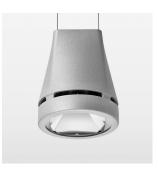
Suspended luminaire with LED, rated life of the LED L80/B10 > 50000 h, colour rendering index CRI > 90, chromaticity tolerance 2 SDCM (initial), reflector with circular light distribution pattern, reflector pure aluminium 99,99% in MIRO-Silver®, canopy sheet steel, powder-coated, luminaire head die-cast aluminium, powder-coated, silver
