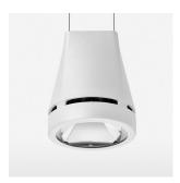
Suspended luminaire with LED, rated life of the LED L80/B10 > 50000 h, colour rendering index CRI > 80, chromaticity tolerance 2 SDCM (initial), reflector with circular light distribution pattern, reflector pure aluminium 99,99% in MIRO-Silver®, canopy sheet steel, powder-coated, luminaire head die-cast aluminium, powder-coated, white
