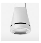
Suspended luminaire with LED, rated life of the LED L80/B10 > 50000 h, colour rendering index CRI > 82, chromaticity tolerance 2 SDCM (initial), reflector with oval light distribution pattern, reflector pure aluminium 99,99% in MIRO-Silver®, luminaire head die-cast aluminium, powder-coated, white
