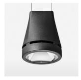
Suspended luminaire with LED, rated life of the LED L80/B10 > 50000 h, colour rendering index CRI > 80, chromaticity tolerance 2 SDCM (initial), reflector with circular light distribution pattern, reflector pure aluminium 99,99% in MIRO-Silver®, luminaire head die-cast aluminium, powder-coated, black, separate driver unit
