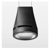
Suspended luminaire with LED, rated life of the LED L80/B10 > 50000 h, colour rendering index CRI > 90, chromaticity tolerance 2 SDCM (initial), reflector with oval light distribution pattern, reflector pure aluminium 99,99% in MIRO-Silver®, luminaire head die-cast aluminium, powder-coated, black
