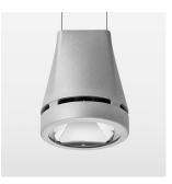
Suspended luminaire with LED, rated life of the LED L80/B10 > 50000 h, colour rendering index CRI > 90, chromaticity tolerance 2 SDCM (initial), reflector with circular light distribution pattern, reflector pure aluminium 99,99% in MIRO-Silver®, luminaire head die-cast aluminium, powder-coated, silver, separate driver unit
