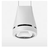
Suspended luminaire with LED, rated life of the LED L80/B10 > 50000 h, colour rendering index CRI > 70, chromaticity tolerance 2 SDCM (initial), reflector with circular light distribution pattern, reflector pure aluminium 99,99% in MIRO-Silver®, luminaire head die-cast aluminium, powder-coated, white, separate driver unit
