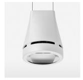
Suspended luminaire with LED, rated life of the LED L80/B10 > 50000 h, colour rendering index CRI > 70, chromaticity tolerance 2 SDCM (initial), reflector with oval light distribution pattern, reflector pure aluminium 99,99% in MIRO-Silver®, canopy sheet steel, powder-coated, luminaire head die-cast aluminium, powder-coated, white
