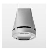
Suspended luminaire with LED, rated life of the LED L80/B10 > 50000 h, colour rendering index CRI > 82, chromaticity tolerance 2 SDCM (initial), reflector with oval light distribution pattern, reflector pure aluminium 99,99% in MIRO-Silver®, canopy sheet steel, powder-coated, luminaire head die-cast aluminium, powder-coated, silver
