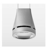
Suspended luminaire with LED, rated life of the LED L80/B10 > 50000 h, colour rendering index CRI > 80, chromaticity tolerance 2 SDCM (initial), reflector with oval light distribution pattern, reflector pure aluminium 99,99% in MIRO-Silver®, luminaire head die-cast aluminium, powder-coated, silver, separate driver unit
