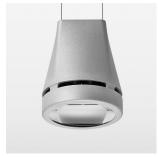
Suspended luminaire with LED, rated life of the LED L80/B10 > 50000 h, colour rendering index CRI > 90, chromaticity tolerance 2 SDCM (initial), reflector with oval light distribution pattern, reflector pure aluminium 99,99% in MIRO-Silver®, luminaire head die-cast aluminium, powder-coated, silver
