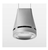
Suspended luminaire with LED, rated life of the LED L80/B10 > 50000 h, colour rendering index CRI > 70, chromaticity tolerance 2 SDCM (initial), reflector with oval light distribution pattern, reflector pure aluminium 99,99% in MIRO-Silver®, canopy sheet steel, powder-coated, luminaire head die-cast aluminium, powder-coated, silver
