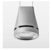
Suspended luminaire with LED, rated life of the LED L80/B10 > 50000 h, colour rendering index CRI > 80, chromaticity tolerance 2 SDCM (initial), reflector with oval light distribution pattern, reflector pure aluminium 99,99% in MIRO-Silver®, canopy sheet steel, powder-coated, luminaire head die-cast aluminium, powder-coated, silver
