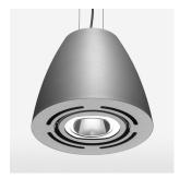
Suspended luminaire with LED, rated life of the LED L80/B10 > 50000 h, colour rendering index CRI > 90, chromaticity tolerance 2 SDCM (initial), reflector with circular light distribution pattern, reflector pure aluminium 99,99% in MIRO-Silver®, swivel angle +/-25°, luminaire housing sheet steel, powder-coated, silver
