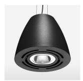
Suspended luminaire with LED, rated life of the LED L80/B10 > 50000 h, colour rendering index CRI > 80, chromaticity tolerance 3 SDCM (initial), reflector with oval light distribution pattern, reflector pure aluminium 99,99% in MIRO-Silver®, swivel angle +/-25°, luminaire housing sheet steel, powder-coated, black
