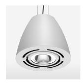
Suspended luminaire with LED, rated life of the LED L80/B10 > 50000 h, colour rendering index CRI > 80, chromaticity tolerance 2 SDCM (initial), reflector with oval light distribution pattern, reflector pure aluminium 99,99% in MIRO-Silver®, swivel angle +/-25°, luminaire housing sheet steel, powder-coated, white
