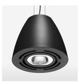
Suspended luminaire with LED, rated life of the LED L80/B10 > 50000 h, colour rendering index CRI > 80, chromaticity tolerance 3 SDCM (initial), reflector with circular light distribution pattern, reflector pure aluminium 99,99% in MIRO-Silver®, swivel angle +/-25°, luminaire housing sheet steel, powder-coated, black
