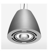
Suspended luminaire with LED, rated life of the LED L80/B10 > 50000 h, colour rendering index CRI > 80, chromaticity tolerance 2 SDCM (initial), reflector with oval light distribution pattern, reflector pure aluminium 99,99% in MIRO-Silver®, swivel angle +/-25°, luminaire housing sheet steel, powder-coated, silver
