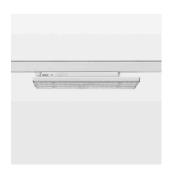
Surface-mounted luminaire with LED, rated life of the LED L90/B50 50000 h (tambient 25°C), colour rendering index CRI > 80, chromaticity tolerance 3 SDCM (initial), extra wide, homogeneous light distribution pattern (90°), TIR-lens made of PMMA, luminaire housing sheet steel, powder-coated, white, locking mechanism to aligned in 15° steps, rotation angle 300°, In-Track-Adapter, Casambi, On/Off, 220-240 V~ / 50-60 Hz, max. 64 luminaires per circuit (B16A fuse)
