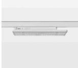
Surface-mounted luminaire with LED, rated life of the LED L90/B50 50000 h (tambient 25°C), colour rendering index CRI > 80, chromaticity tolerance 3 SDCM (initial), wide, homogeneous light distribution pattern (60°), TIR-lens made of PMMA, luminaire housing sheet steel, powder-coated, white, locking mechanism to aligned in 15° steps, rotation angle 300°, In-Track-Adapter, Casambi, On/Off, 220-240 V~ / 50-60 Hz, max. 64 luminaires per circuit (B16A fuse)
