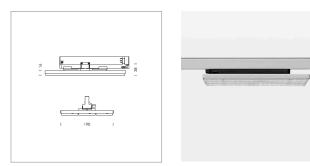
Surface-mounted luminaire with LED, rated life of the LED L90/B50 50000 h (tambient 25°C), colour rendering index CRI > 80, chromaticity tolerance 3 SDCM (initial), wide, homogeneous light distribution pattern 30°, TIR-lens made of PMMA, luminaire housing sheet steel, powder-coated, silver, locking mechanism to aligned in 15° steps, rotation angle 300°, In-Track-Adapter, Casambi, 220-240 V~/ 50-60 Hz, max. 64 luminaires per circuit (B16A fuse)
