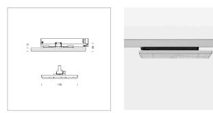
Surface-mounted luminaire with LED, rated life of the LED L90/B50 50000 h (tambient 25°C), colour rendering index CRI > 80, chromaticity tolerance 3 SDCM (initial), wide, homogeneous light distribution pattern 30°, TIR-lens made of PMMA, luminaire housing sheet steel, powder-coated, silver, locking mechanism to aligned in 15° steps, rotation angle 300°, In-Track-Adapter, Casambi, 220-240 V~/ 50-60 Hz, max. 64 luminaires per circuit (B16A fuse)
