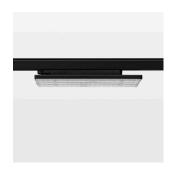
Surface-mounted luminaire with LED, rated life of the LED L90/B50 50000 h (tambient 25°C), colour rendering index CRI > 80, chromaticity tolerance 3 SDCM (initial), wide, homogeneous light distribution pattern 30°, TIR-lens made of PMMA, luminaire housing sheet steel, powder-coated, black, locking mechanism to aligned in 15° steps, rotation angle 300°, In-Track-Adapter, Casambi, 220-240 V~ / 50-60 Hz, max. 64 luminaires per circuit (B16A fuse)
