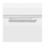
Surface-mounted luminaire with LED, rated life of the LED L90/B50 50000 h (tambient 25°C), colour rendering index CRI > 80, chromaticity tolerance 3 SDCM (initial), extra wide, homogeneous light distribution pattern (90°), TIR-lens made of PMMA, luminaire housing sheet steel, powder-coated, white, locking mechanism to aligned in 15° steps, rotation angle 300°, In-Track-Adapter, On/Off, 220-240 V~ / 50-60 Hz, max. 27 luminaires per circuit (B16A fuse)
