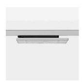
Surface-mounted luminaire with LED, rated life of the LED L90/B50 50000 h (tambient 25°C), colour rendering index CRI > 80, chromaticity tolerance 3 SDCM (initial), extra wide, homogeneous light distribution pattern (90°), TIR-lens made of PMMA, luminaire housing sheet steel, powder-coated, silver, locking mechanism to aligned in 15° steps, rotation angle 300°, In-Track-Adapter, On/Off, 220-240 V~ / 50-60 Hz, max. 27 luminaires per circuit (B16A fuse)
