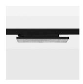
Surface-mounted luminaire with LED, rated life of the LED L90/B50 50000 h (tambient 25°C), colour rendering index CRI > 80, chromaticity tolerance 3 SDCM (initial), extra wide, homogeneous light distribution pattern (90°), TIR-lens made of PMMA, luminaire housing sheet steel, powder-coated, black, locking mechanism to aligned in 15° steps, rotation angle 300°, In-Track-Adapter, On/Off, 220-240 V~ / 50-60 Hz, max. 27 luminaires per circuit (B16A fuse)
