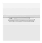
Surface-mounted luminaire with LED, rated life of the LED L90/B50 50000 h (tambient 25°C), colour rendering index CRI > 80, chromaticity tolerance 3 SDCM (initial), wide, homogeneous light distribution pattern (60°), TIR-lens made of PMMA, luminaire housing sheet steel, powder-coated, white, locking mechanism to aligned in 15° steps, rotation angle 300°, In-Track-Adapter, On/Off, 220-240 V~ / 50-60 Hz, max. 27 luminaires per circuit (B16A fuse)
