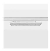
Surface-mounted luminaire with LED, rated life of the LED L90/B50 50000 h (tambient 25°C), colour rendering index CRI > 80, chromaticity tolerance 3 SDCM (initial), wide, homogeneous light distribution pattern 30°, TIR-lens made of PMMA, luminaire housing sheet steel, powder-coated, white, locking mechanism to aligned in 15° steps, rotation angle 300°, In-Track-Adapter, On/Off, 220-240 V~ / 50-60 Hz, max. 27 luminaires per circuit (B16A fuse)
